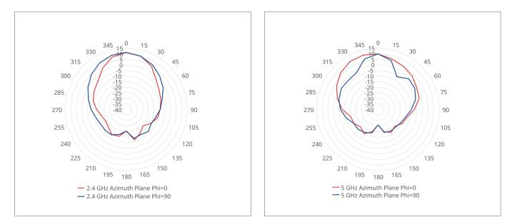
The following figures shows the elevation antenna pattern at 2.4 GHz and 5 GHz radios.
